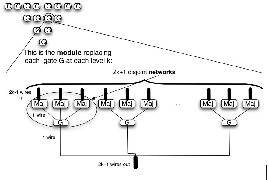
We say a **network** errs if the wire leaving it has a different value than the wire leaving the corresponding gate, G, in the noiseless circuit. Say the entire **module** errs if a majority of the wires leaving it differ from wire leaving the corresponding G in the noiseless circuit
